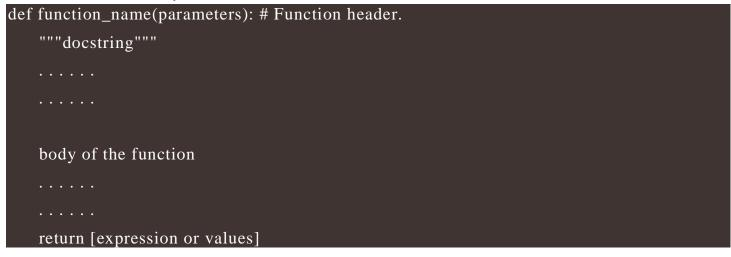
In the above syntax, the first line of function definition is header, and the rest is the body of function. The function definition begins with def keyword followed by the function
